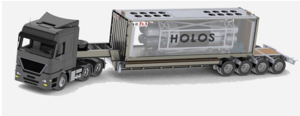
Figure 1.1 Rendering of the HolosGen Holos Reactor Shipping (HolosGen, 2017)
