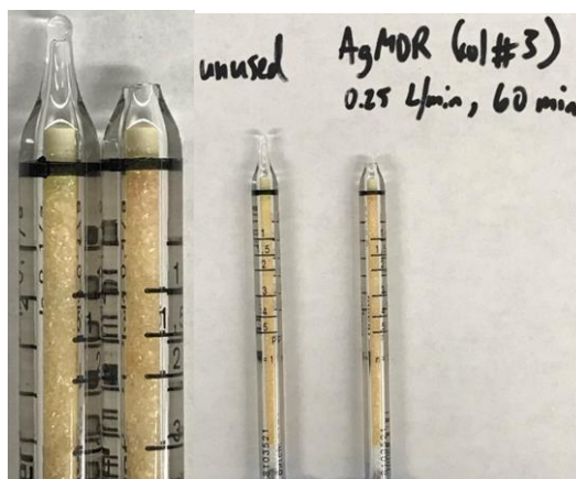
Figure 52: Draeger tube analysis for fully exchanged silver mordenite
