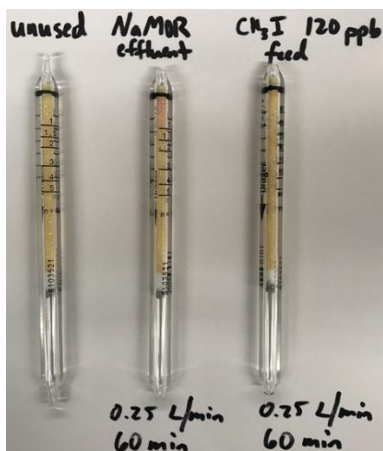
Figure 50: Draeger tube analysis for sodium mordenite
