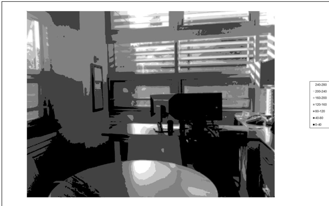
Figure 1.30 Site for Glazing Installation: 2pm glare in Southwest wing of building and site of future View Dynamic Glass installation; Probert 2013
