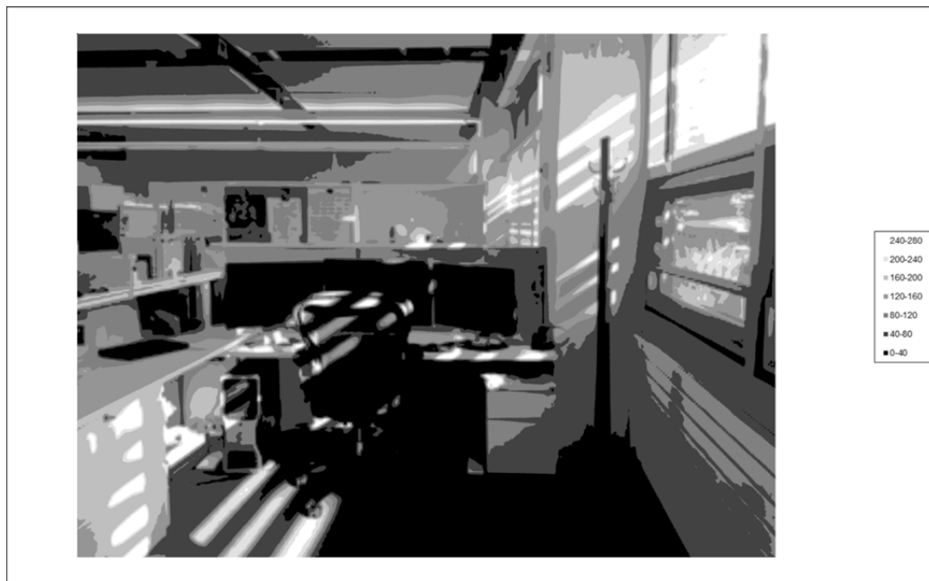
Figure 1.26 Glare Due to Shading Calibration Problems: Contrast glare and intermittent direct sun glare occurred in the South-facing North wing of the first floor of the building because Mecchoshades were not responding to direct sun; Probert 2013
