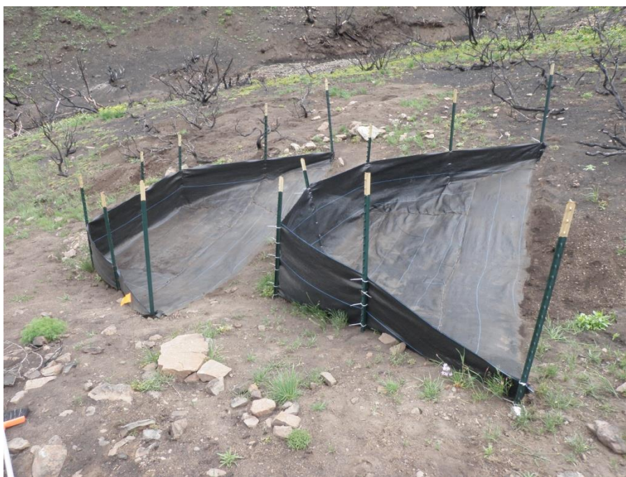
Figure 2.10. Image of a swale plot showing how the two silt fences are placed as the downslope base.
