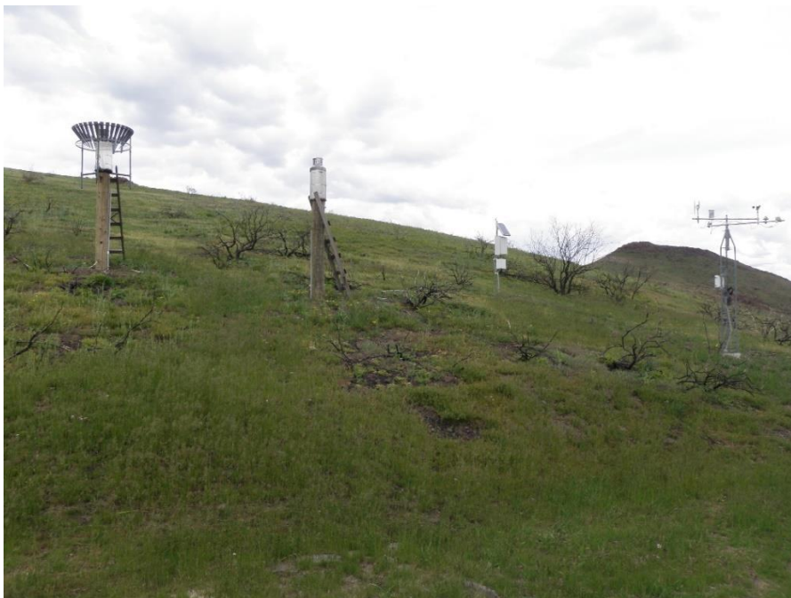
Figure 2.6. Image of the USDA-ARS-NWRC meteorological station, Murphy Creek (site# 043) located at the base of the watershed. The meteorological station measures hourly precipitation, temperature, relative humidity, wind, and solar radiation.
