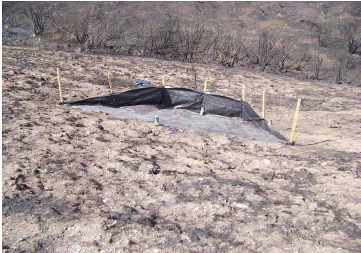
Figure 1.1. Silt fences are used as a method to measure hillslope erosion. This silt fence was assembled using synthetic geotextile, wooden posts to stabilize the fence, and sod staples to secure the silt fence to the ground surface.
