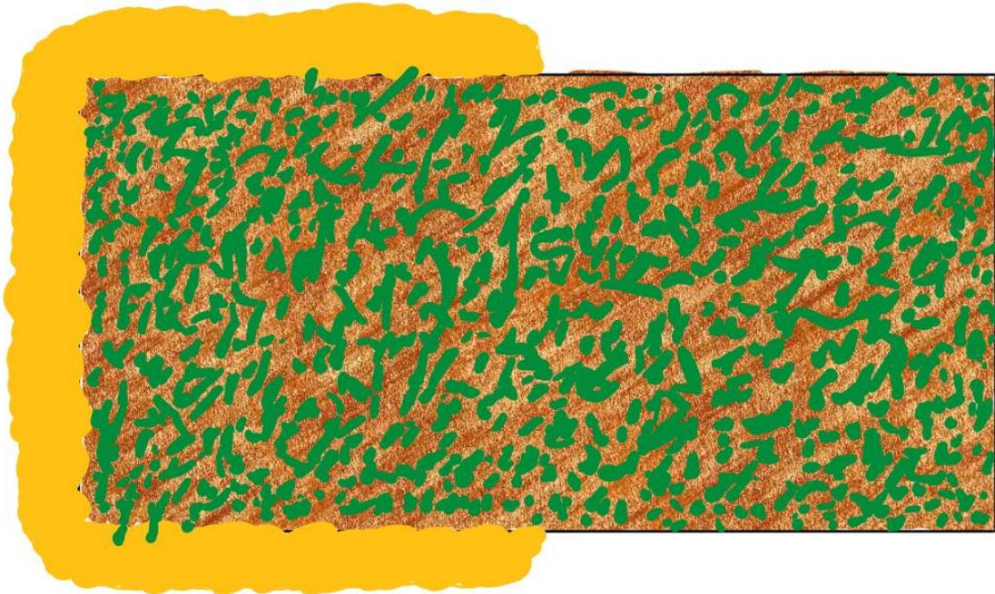
Figure 2. 1. Schematic of the burning setup with the horseshoe-shaped ignition fuel configuration. Yellow- excelsior; brown- soil, green- grass (fuel load), black- tray edge.
