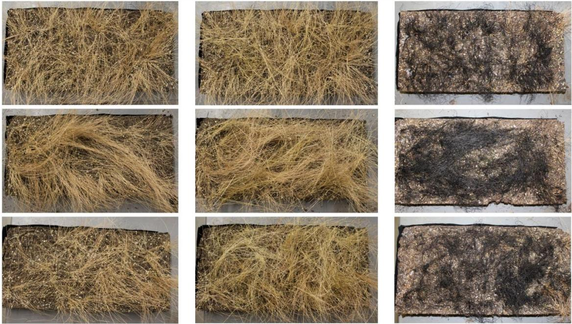
Figure A. 4. FEID burning patterns. From left to right: FEID without BRTE (natural fuel load), FEID with added BRTE, after burning. From up to the bottom: 20 % of BRTE added, 50 % of BRTE added, 80 % of BRTE added.
