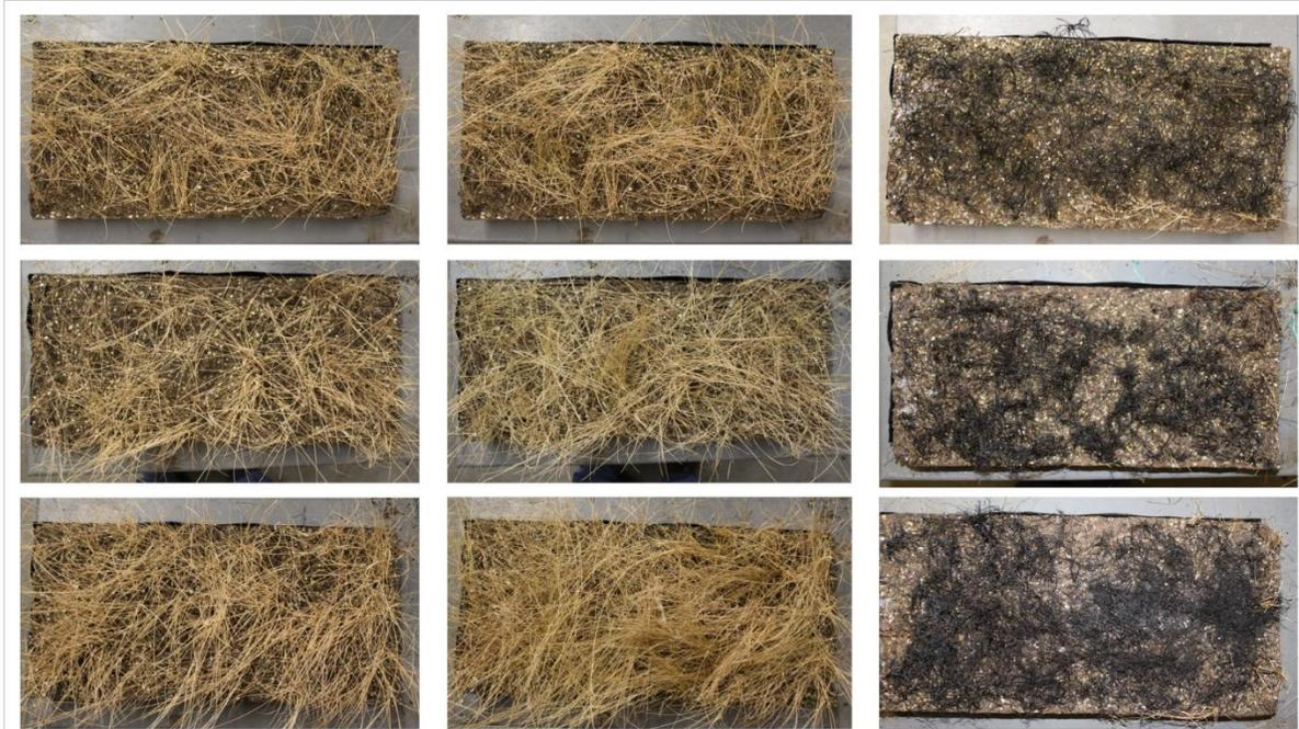
*Figure A. 3. PSSP burning patterns. From left to right: PSSP without BRTE (natural fuel load), PSSP with added BRTE, after burning. From up to the bottom: 20% BRTE added, 50% BRTE added, 80% BRTE added.*
