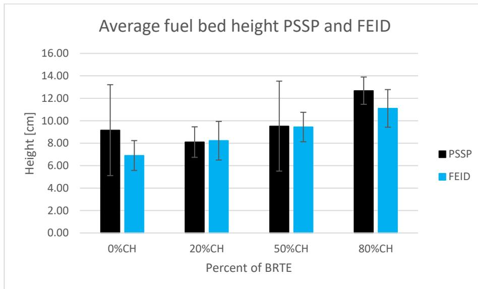
Figure 3. 4. Average fuel height for PSSP and FEID in relation to fuel addition in percent of BRTE added.
