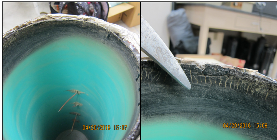
Figure 1.9: Damage to the PVC pipe from the 1 st experiment.
