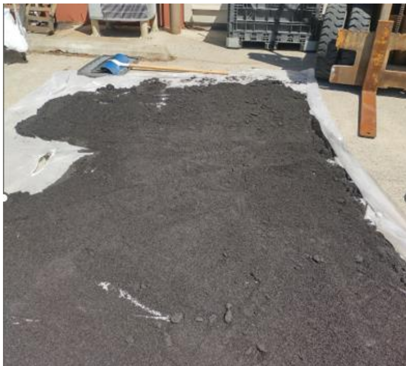
Figure 23. Picture of pilot scale Fe-modified biochar drying after modification process.
