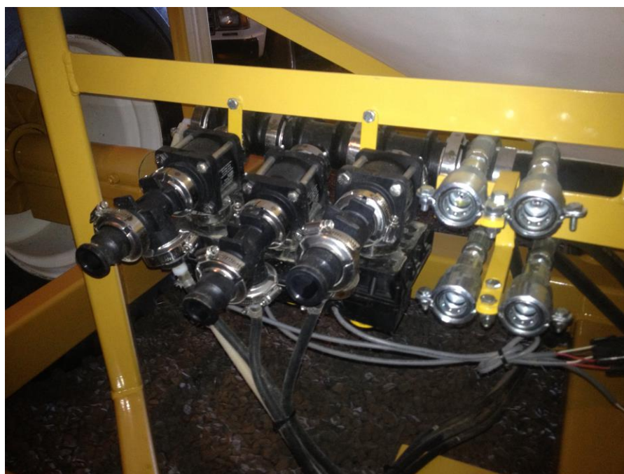
Figure 26. Three valve system to vary application rate in three sections of the cultivator.
