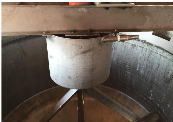
Figure 72 - Plant Pilot Thickener Feed Well
