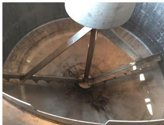
Figure 73 - Plant Pilot Thickener Rake
