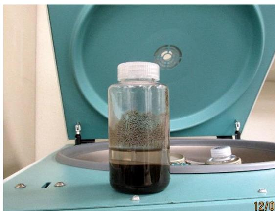
Figure 10 - Sample after Centrifuging
