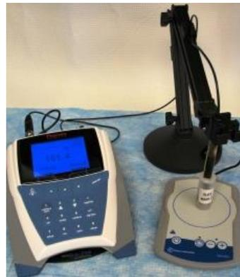
Figure 22 - Thermo/Orion Fluoride Probe
