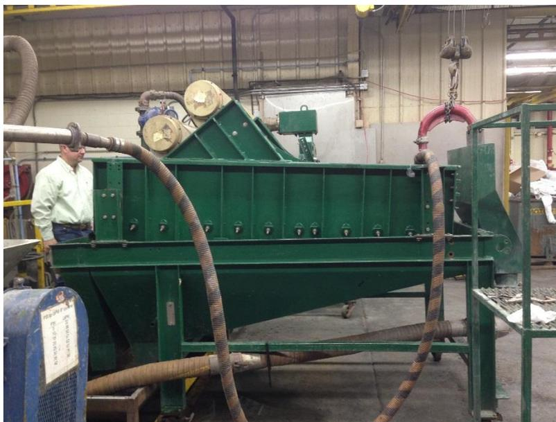
Figure 74 - Dewatering Screen Side View
