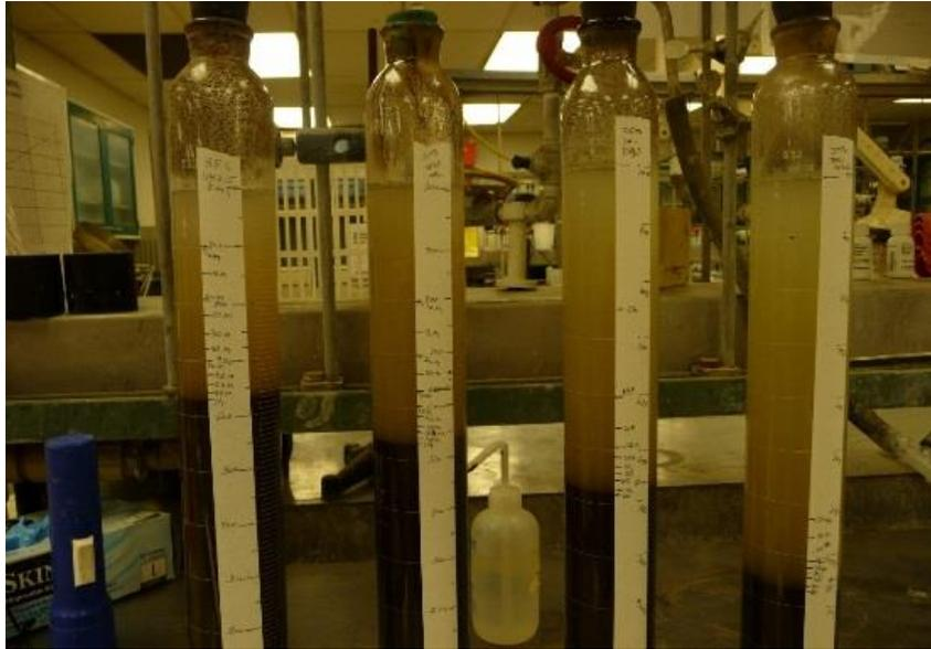
Figure 14 - Sedimentation Cylinders
