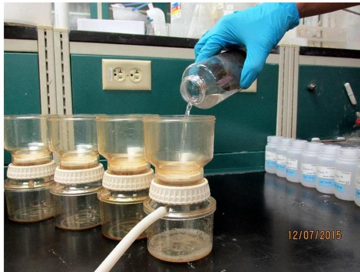
Figure 12 - Vacuum Filtration of Supernatant
