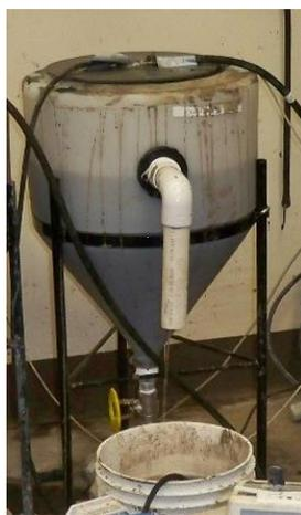
Figure 71 - Lab Pilot Conical Thickener
