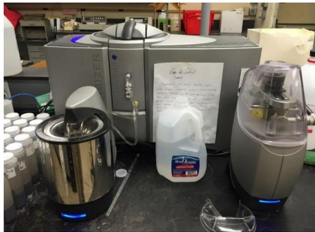
Figure 23 - Malvern Particle Size Analyzer
