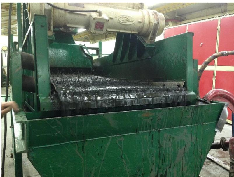
Figure 75 - Dewatering Screen Solids Discharge
