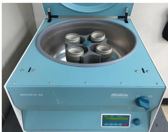
Figure 9 - Lab Centrifuge
