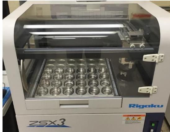
Figure 20 - Rigaku XRF Analyzer
