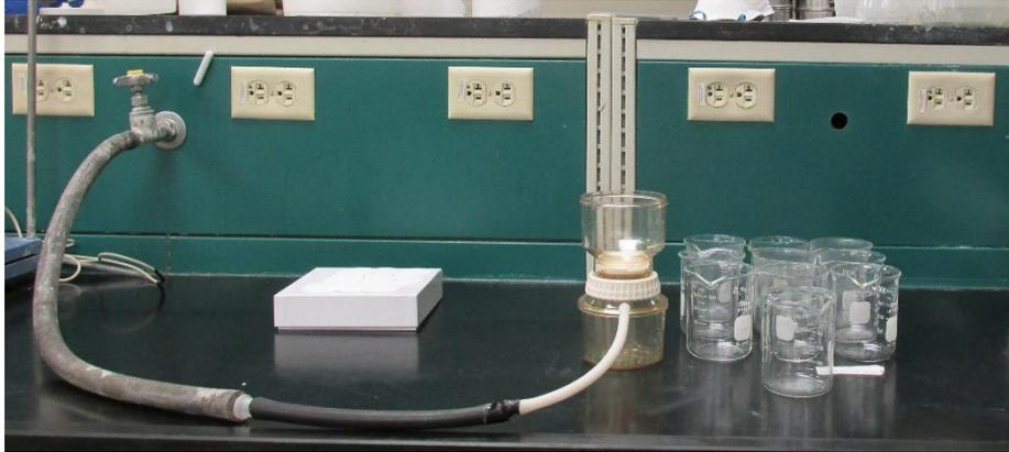
Figure 11 - Vacuum Filtration Apparatus
