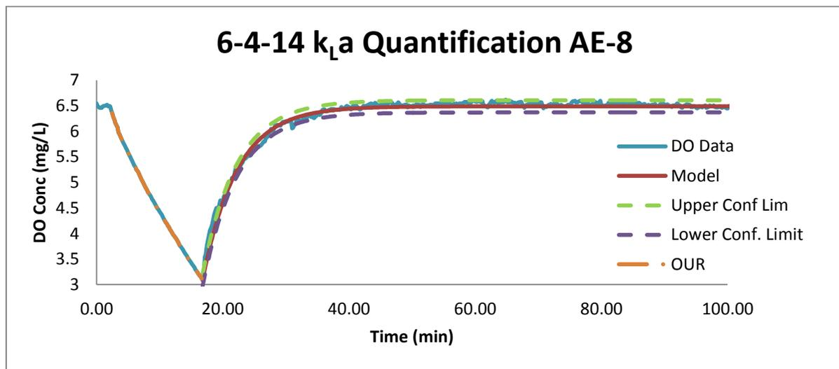
Figure 15: Example  $k_La$  Fitting Model.
