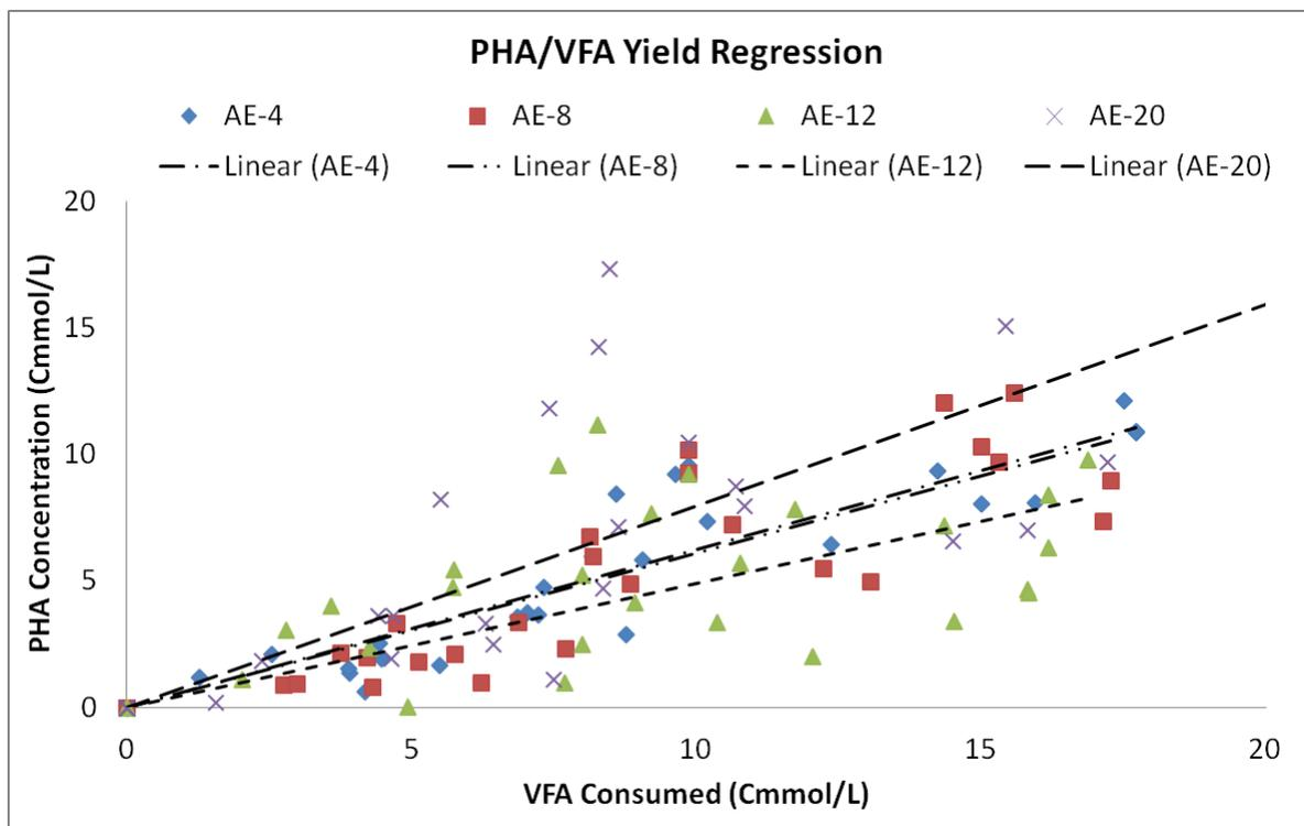
Figure 27: Regression results and data, used to model reactor Enrichment yield (PHA/VFA).
