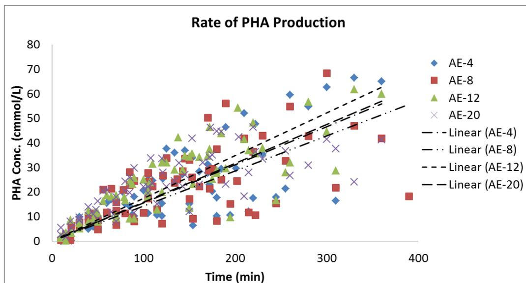
Figure 38: Rate of PHA Synthesis, linear regression and data.
