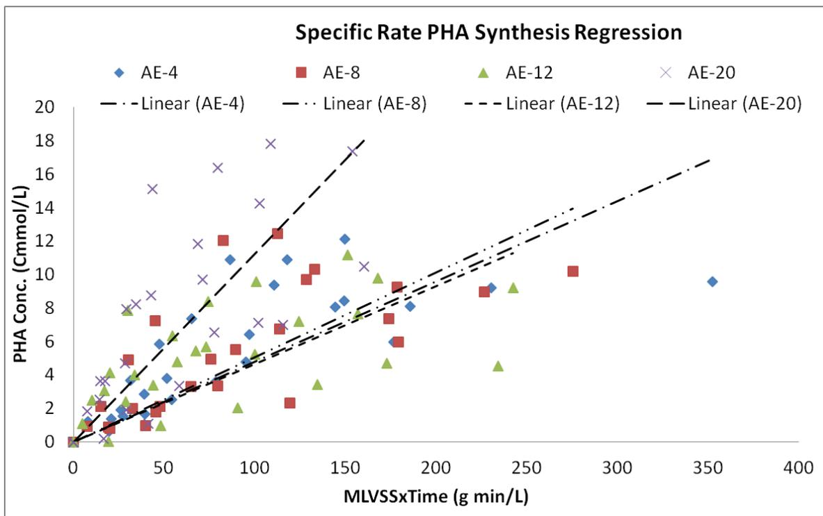
Figure 30: Enrichment evaluation PHA synthesis models.
