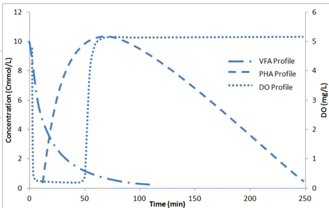
Figure 18: Idealized "Typical" enrichment reactor data.
