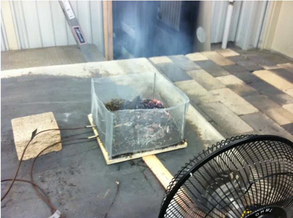
Figure 11 Final combustion/consumption container and fan setup for lab experimentation
