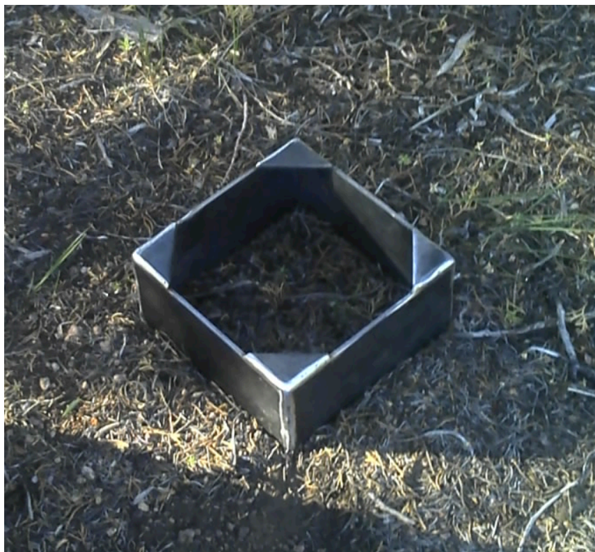
Figure 10 20x20 cm steel frame used to extract duff samples for lab experimentation
