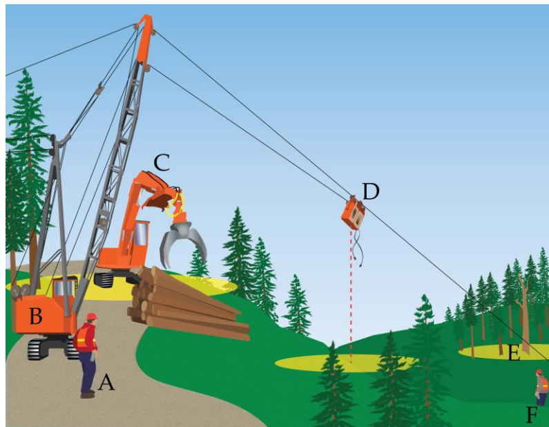
Figure 2.3. Typical cable logging operation with (A) chaser, (B) yarder, (C) loader, (D) carriage, (E) snag, and (F) hooker (note: images are not drawn to scale). Yellow ellipses highlight areas with increased risk of injury associated with the three types of hazards shown. Of the three hazards, snag GNSS coordinates were fixed (static), while loader and carriage locations were dynamic.
