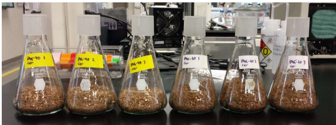
Figure A.3. Corn stover inoculated with C. subvermispora after 2 weeks of storage. 40% moisture content samples are on the left, and 60% moisture content samples are on the right.
