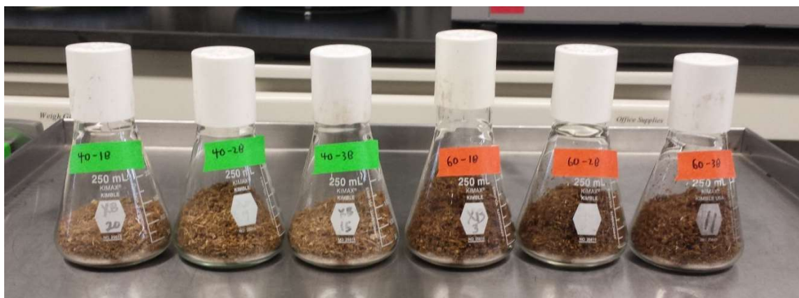
Figure A.2. Corn stover with no inoculum after 2 weeks of storage. 40% moisture content samples are on the left, and 60% moisture content samples are on the right.
