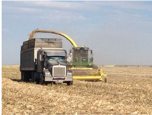
Figure 1.7 Collection of corn stover with forage chopper into a walking floor trailer.
