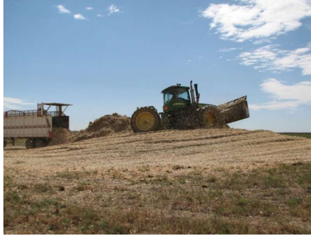
Figure 1.8 Simultaneous formation and compaction of a drive over storage pile with corn stover unloaded from walking floor trailers.
