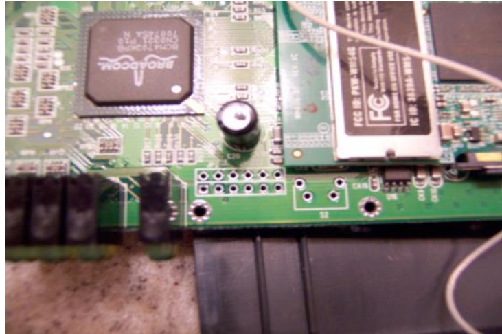
Figure 3-6: Unpopulated JTAG connector on a DD WRT router [32]
