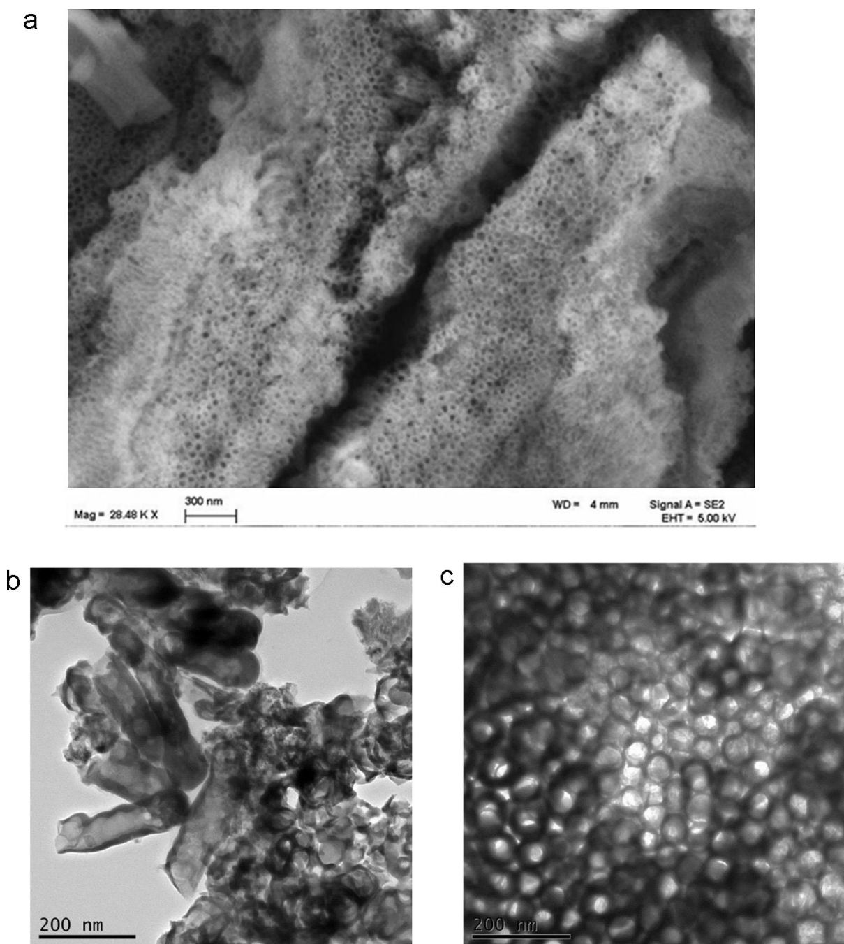
Figure 3.3: Electron microscopic images of oxide layers formed on the Zr–W alloy substrate after anodization at 40 V for 1 h in EG electrolyte containing 0.2 M \text{NH}_4\text{F} + 5 vol% \text{H}_2\text{O} . (a) FESEM image of the top surface of the anodic oxide layer revealing nanotubular morphology;
