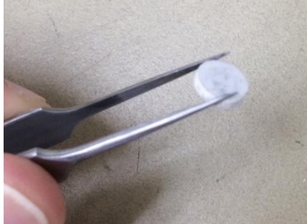
Figure 1.33: Incomplete pellet of \text{LaNbO}_4 after pressing process
