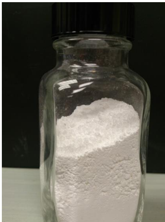
Figure 1.30: Photograph of synthesized lanthanum niobate powder
