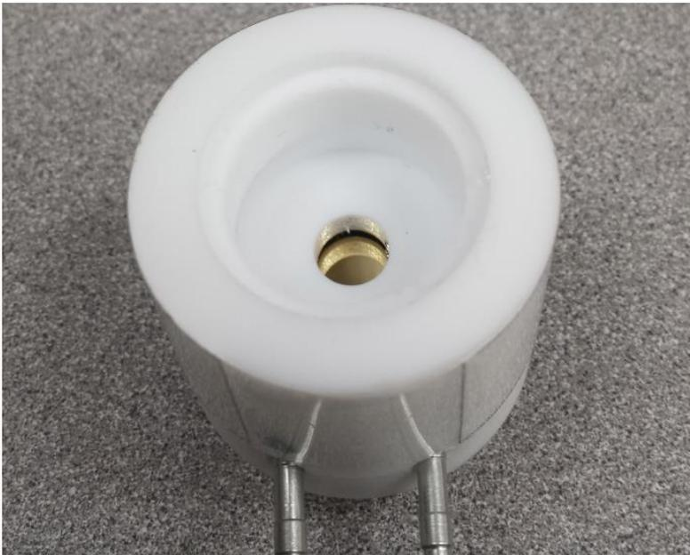
**Figure 49: QCM submerged in water cell (open top)**
