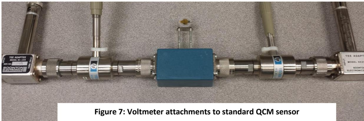
**Figure 7: Voltmeter attachments to standard QCM sensor**
