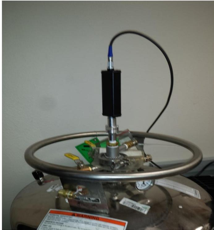
**Figure 10: Data collection head attached to 100L helium dewar**
