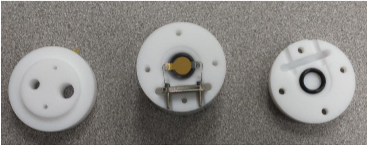
**Figure 48: QCM resting in disassembled cell**
