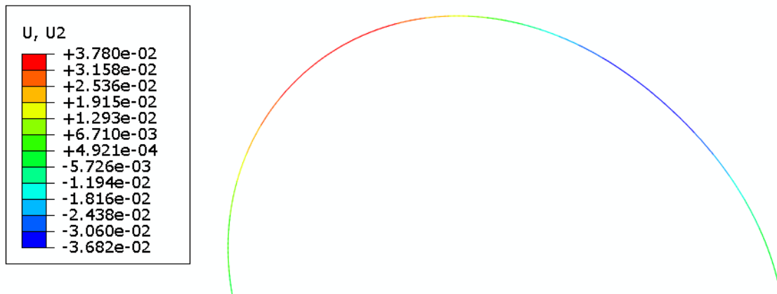
Figure 6-14 Case 7 Abaqus Vertical Deflection
