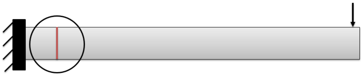
Figure 2-9 Cross Section in Inelastic Bending
