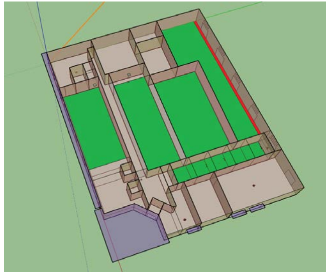
Figure 4.5: An illustration of the CSHQA floorplan from the OpenStudio plug-in for SketchUp.
