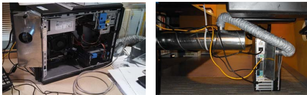
Figure 4.3: The computer exhaust system developed by Russ Pratt [40] [80].
