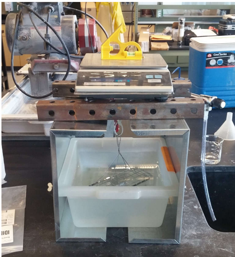
Figure C.1. Denver Instrument XL6100 scale modified to make saturated mass measurements.
