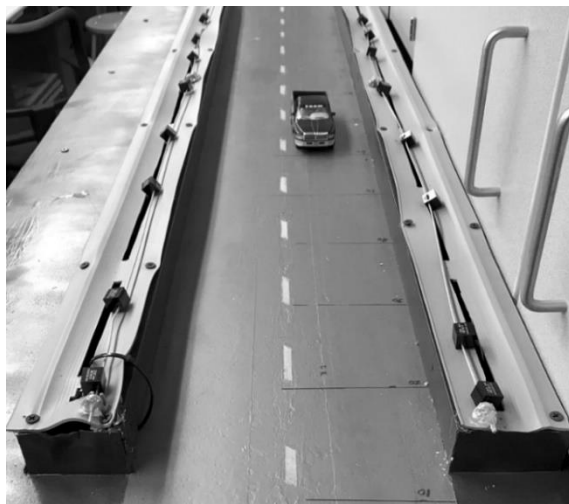
Figure 7-27. Two-lane straight road model with model vehicle for TZOID image sensor testing.
