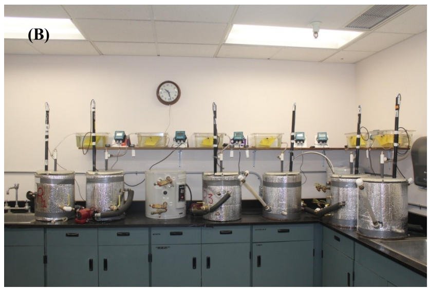
Fig. 3.1 - Schematic of anaerobic digester and a picture of the anaerobic digesters in a laboratory setup (A) schematic of anaerobic digester, (B) picture of six anaerobic digesters used for anaerobic digestion test.
