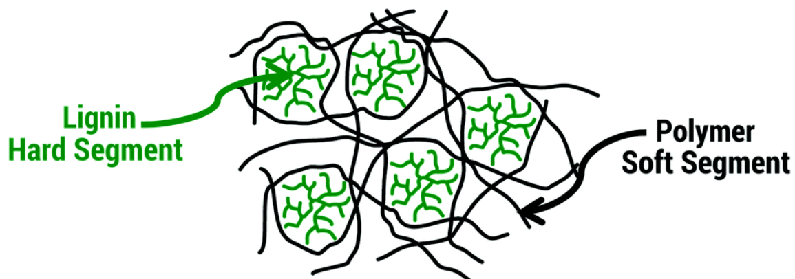
Figure 1.2 Hard and soft segments of lignin copolymers taken from Bova, et al., 2016
