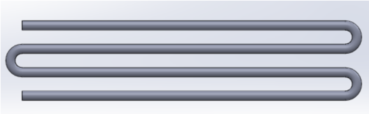
Figure 3.3: Simplified version of a single tube within the tube bank.
