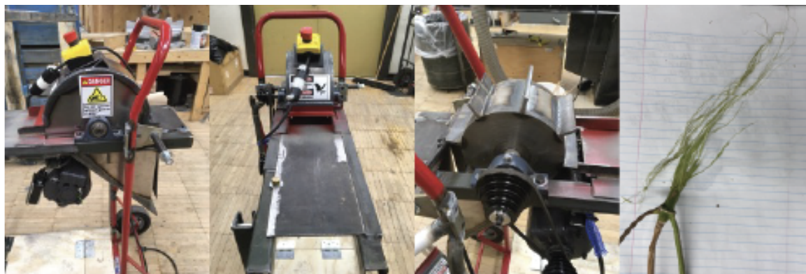
Figure 3.1 Lab-scaled decortication machine with an example of fiber separation from the beating roller.
