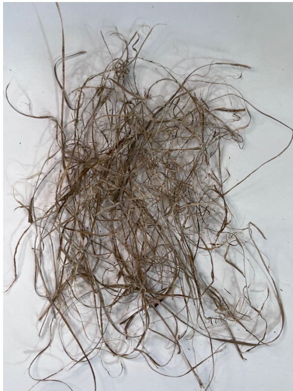
Figure 4.3 Breaking to water retted fibers.
