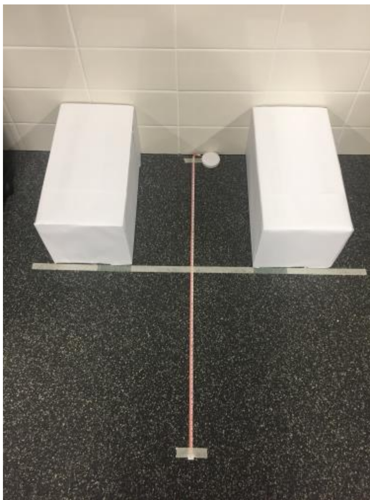
Figure 3.1: Setup of the V-SR with two tape boxes, Medco® Sports Medicine cloth tape measure (150cm), and Duck® Tape Beige General Purpose Masking Tape (18mm X 55m)
