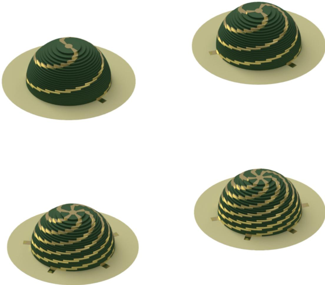
Figure 4.2: Two, three, five, and six arm hemispherical helix antennas created using a stack of 24 PCBs.
