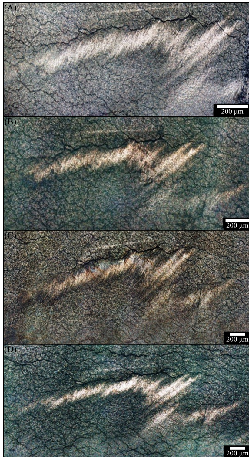
Figure 4.11: Micrograph of FSP 304L+316L sample after (A): 102.75 hours (B): 127 hours (C): 152.75 hours (D): 174 hours
