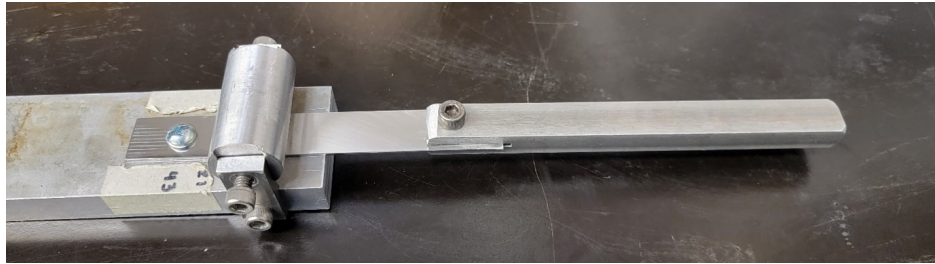
Figure 4.5: Jig used to repeatedly bend samples to the correct size
