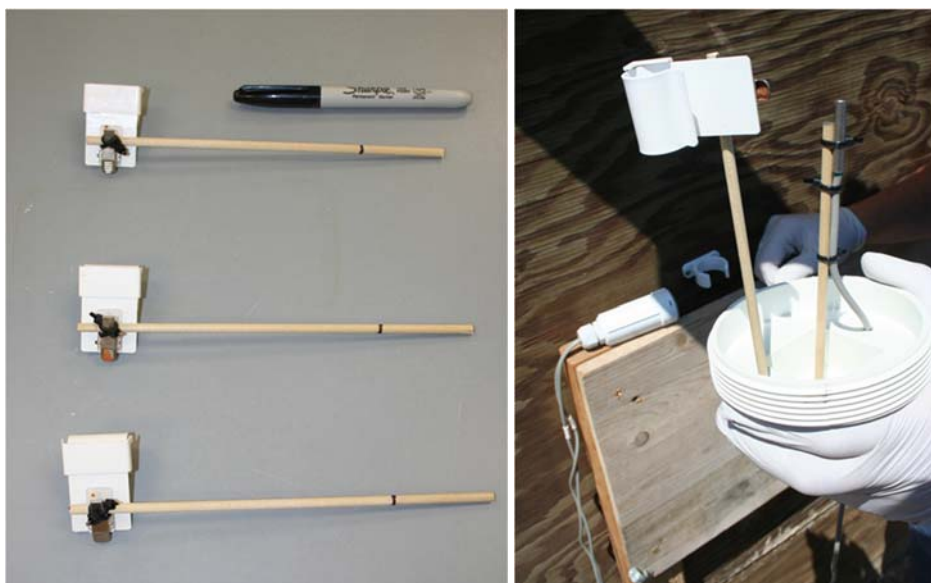
Picture 4. 10 Ogawa samplers holders and sampling port insertion
