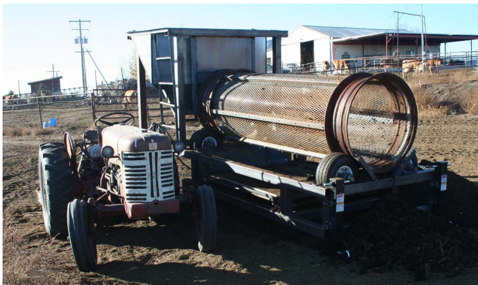
Picture 4. 31 Compost screen operating connected to an older tractor
