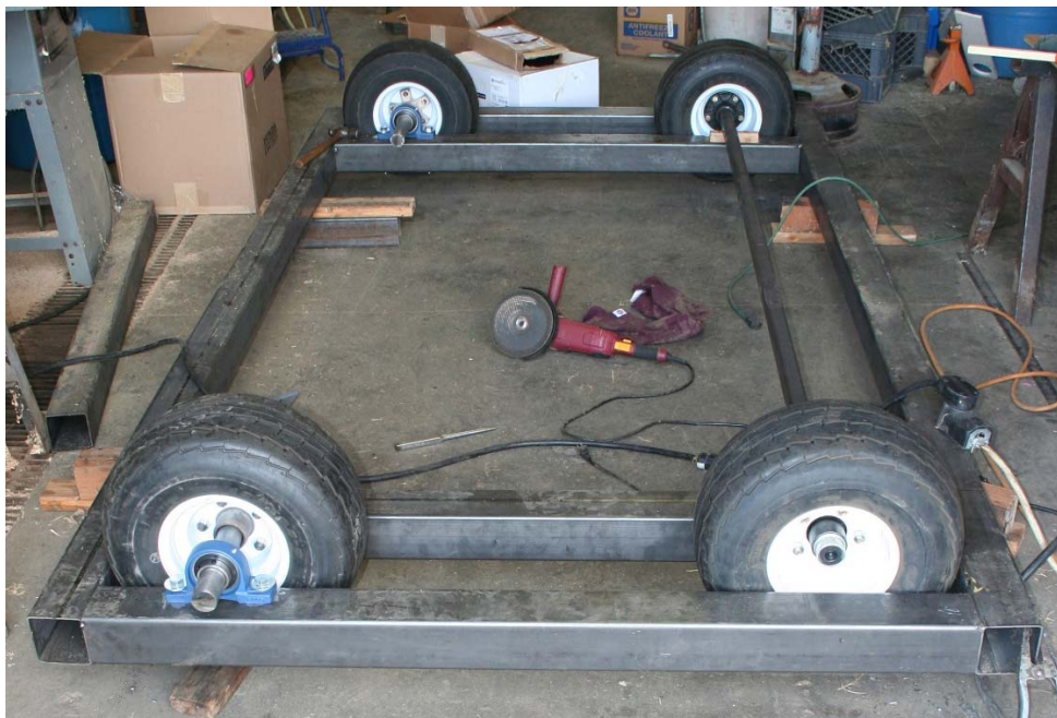
Picture 4. 22 Compost screen chassis and screen holding wheels
