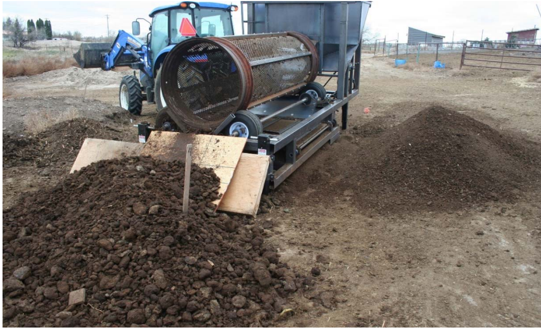
Picture 4. 27 View of rotatory screen powered by tractor's hydraulics
