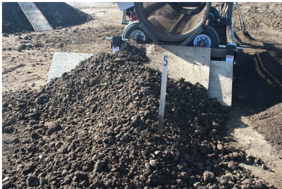
Figure 2. 14 Refuse from screening
