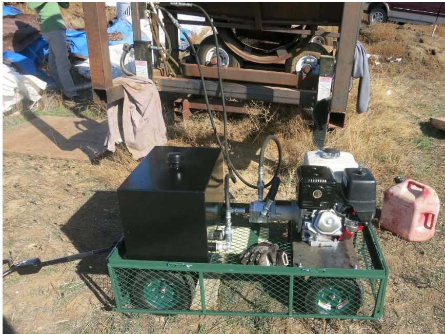
Picture 4. 28 Small engine, hydraulic pump and oil reservoir on a cart
