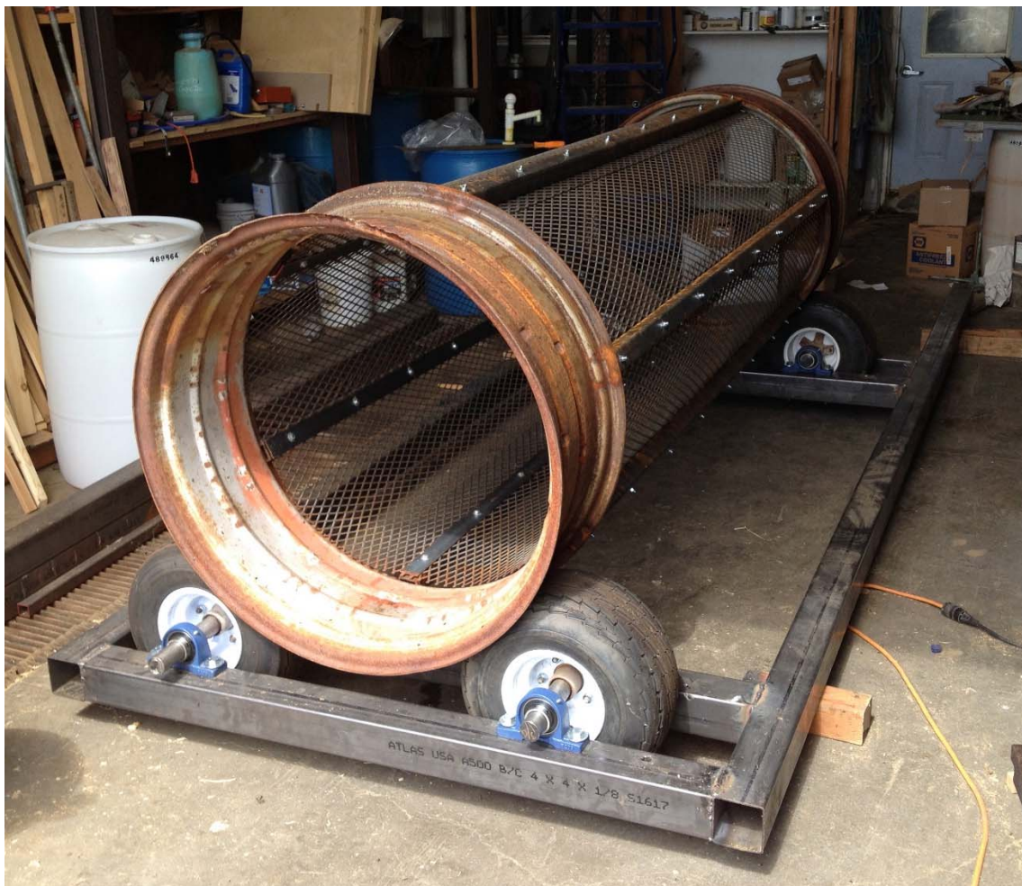
Picture 4. 24 Screen drum mounted over wheels and chassis
