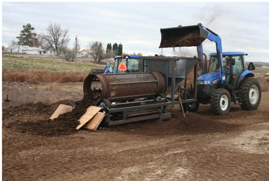
Figure 2. 10 Compost screening using custom made rotatory screen
