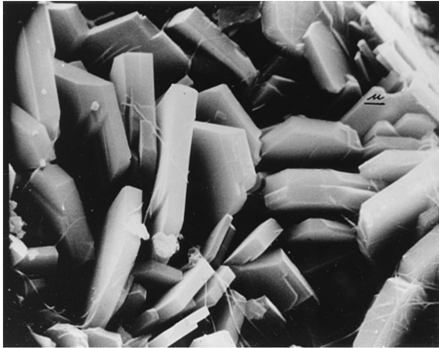
Picture 1. 1 Scanning electron micrograph of plates of clinoptilolite from Castle Creek, ID.
