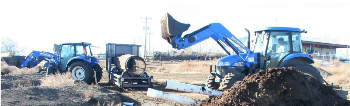
Picture 4. 30 Compost screen operating connected to a tractor
