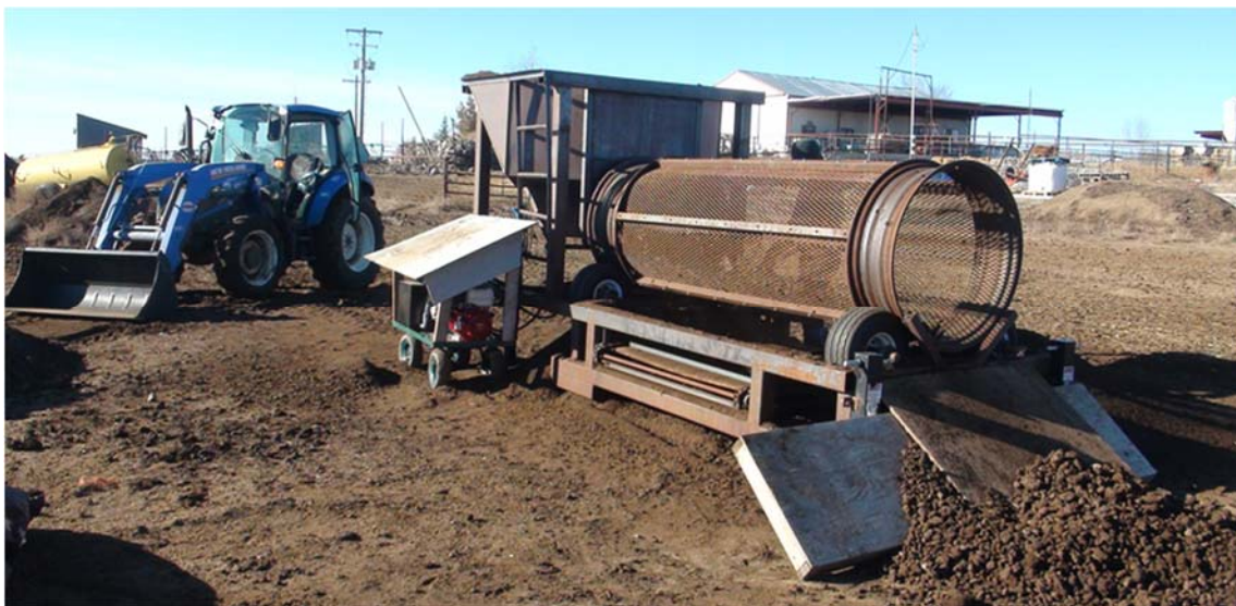
Picture 4. 29 Compost screen with portable engine and pump setting
