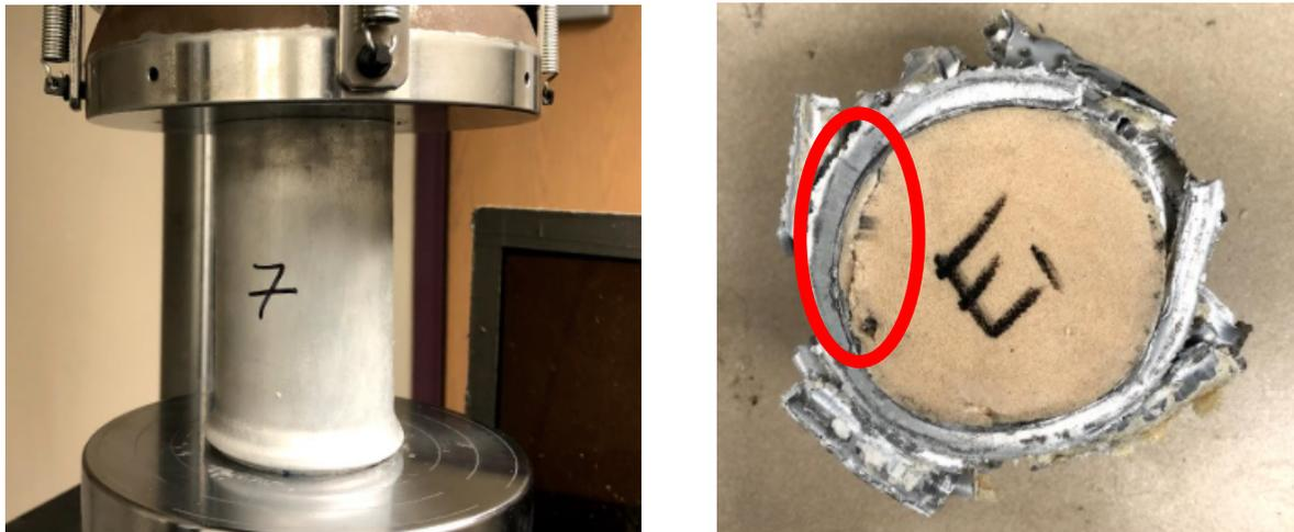
**Figure 4-9: A-FE120 crushing behavior**
