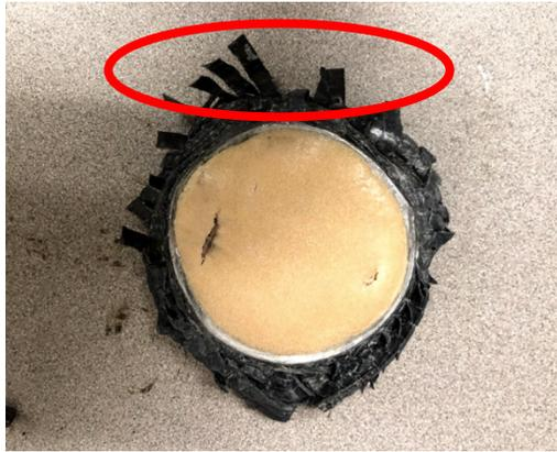
**Figure 2-7: Fronds in CFRP reinforced tubes**
