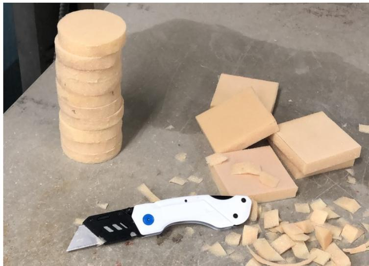
Figure 3-7: PVC foam cut into circles and squares
