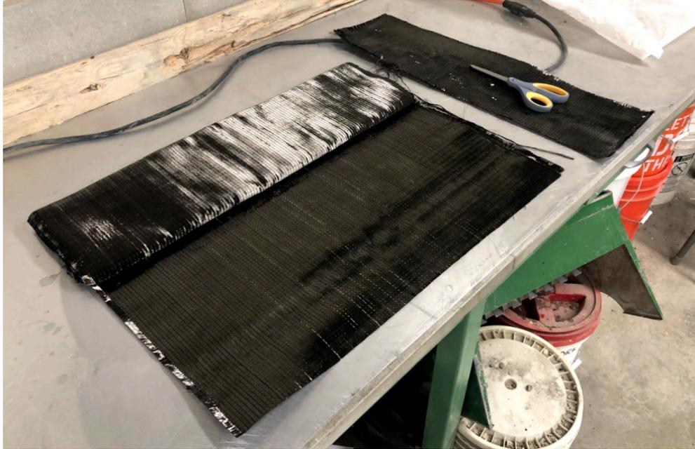
**Figure 3-4: Carbon fiber unidirectional sheet**
