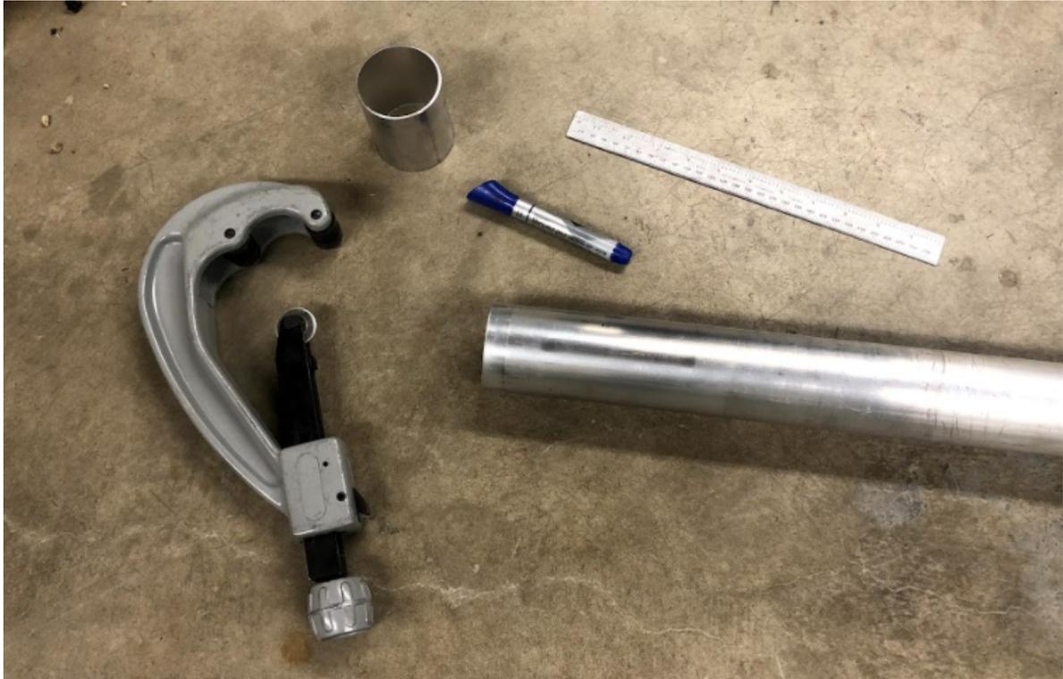
Figure 3-3: Cutting equipment for aluminum tubes
