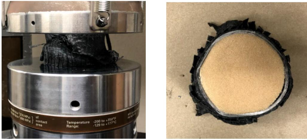
Figure 4-13: C-F80 crushing behavior
