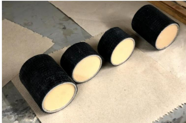
**Figure 3-8: C-F80 and C-F40 tubes during curing**
