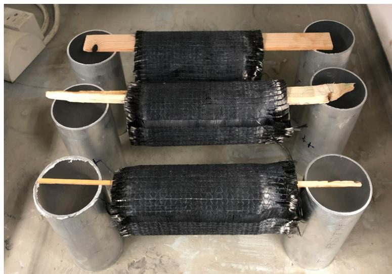
**Figure 3-5: CFRP reinforced samples during curing process**
