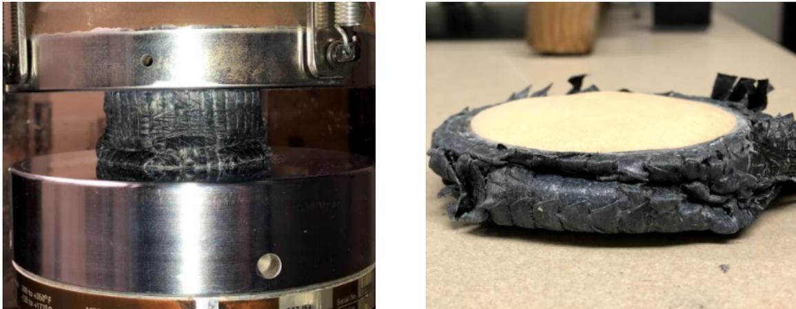
Figure 4-15: C-F40 crushing behavior
