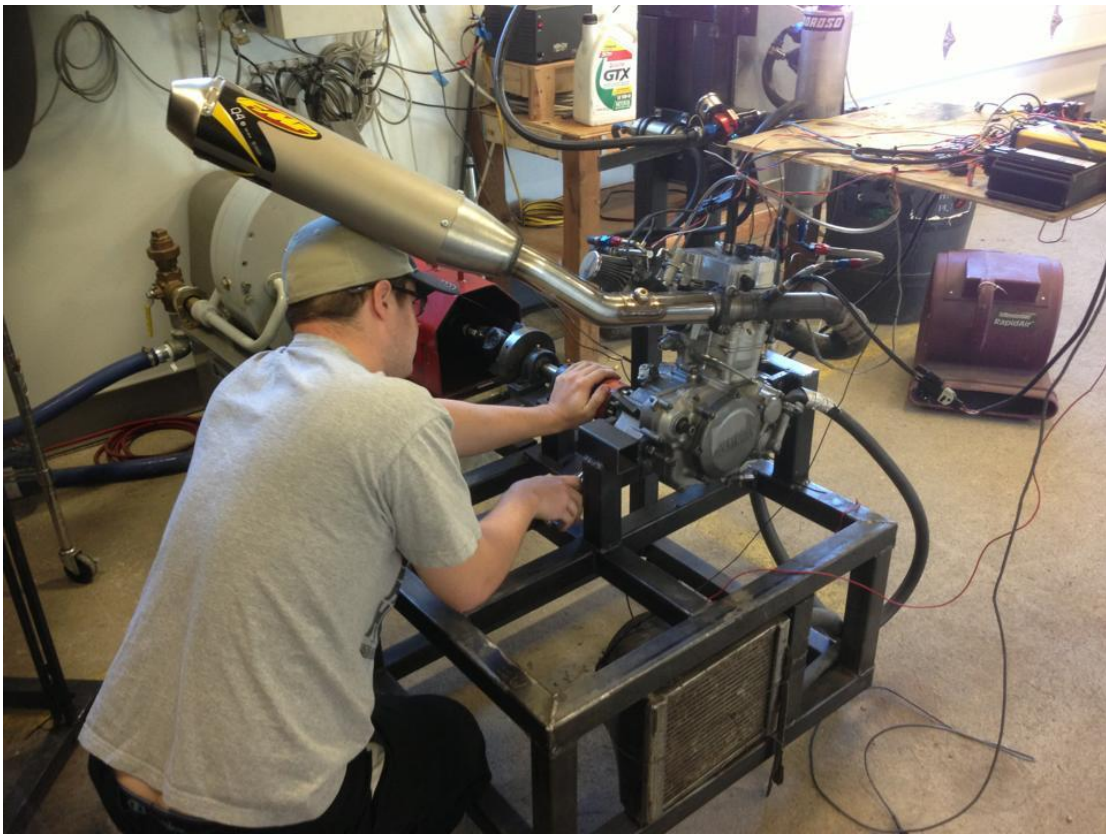
Figure 24: Dynamometer Testing Setup
