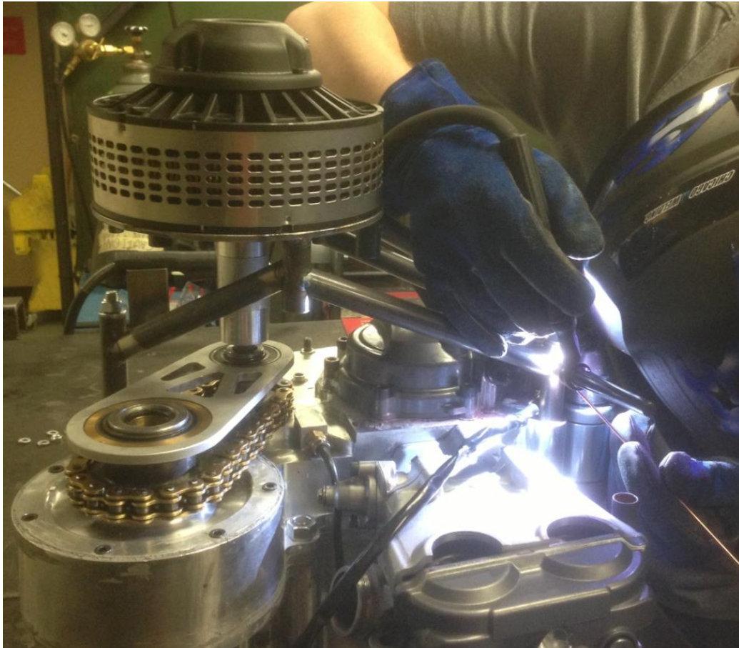
Figure 18: EM Mount Manufacturing – Tack Welding
