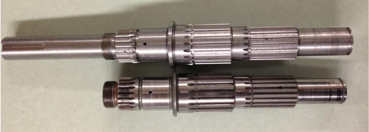
Figure 16: Custom (top) and Stock (bottom) Output Shafts
