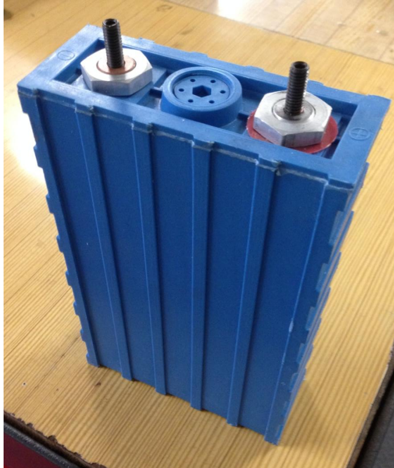
Figure 3: CALB 40 Ah LiFePo Cell
