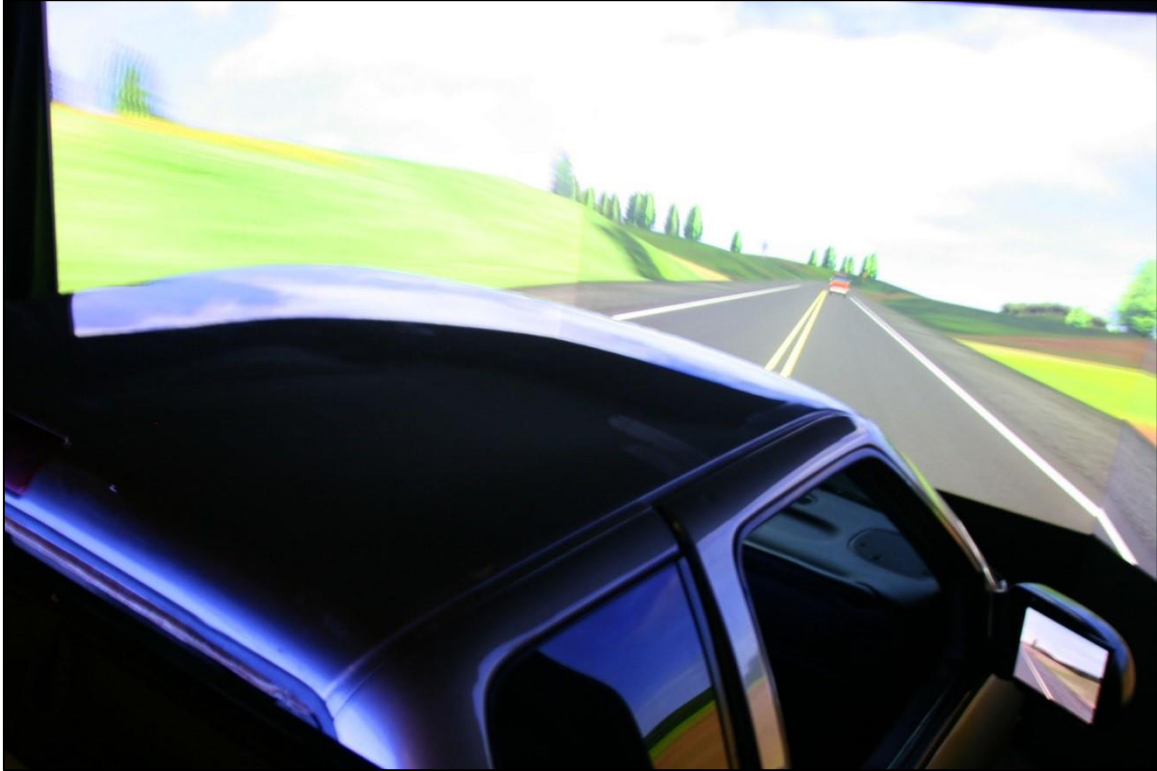
Figure 16: Cab with Projected Screens
