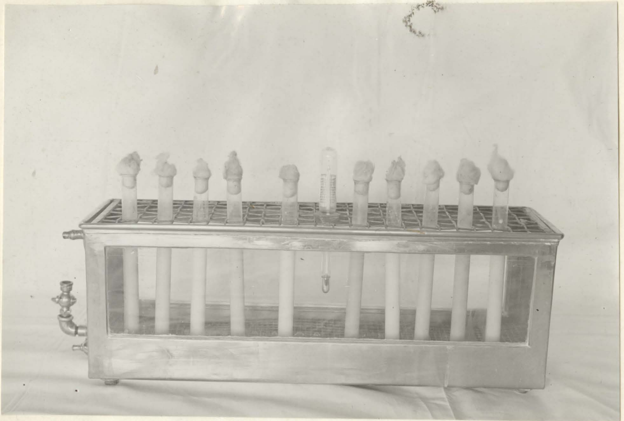
Apparatus used for the methylene blue reduction test.
