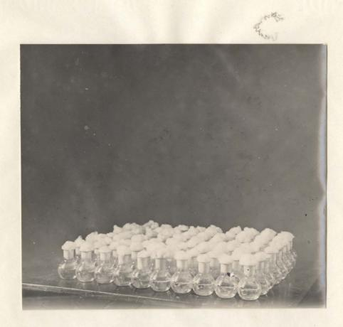
Plate II. Series of flasks inoculated with soil for the formation of nitrites and nitrates.
