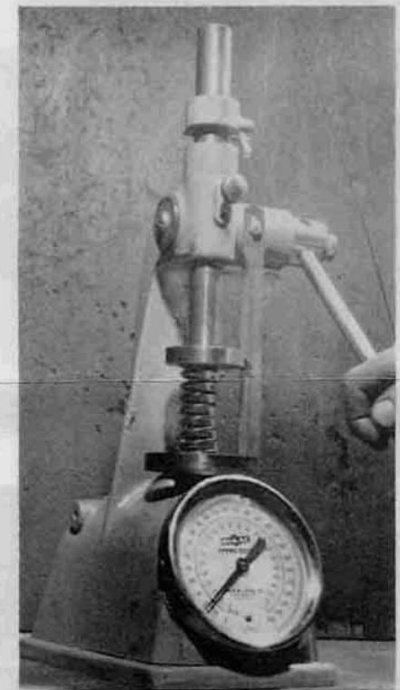
Above—This spring tester measures the strength and length of valve and clutch springs on truck engines. It has corrected much poor engine performance as many engines were found to have weak valve springs. The tester is another modern shop tool now furnished woods mechanics to enable them to do a better repair job.
