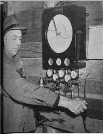
Above—Lyle Williams, Rutledge kiln foreman, has a look at the instruments which control kiln No. 2 at the Coeur d'Alene plant. The clock with its inking needles (or pens) that writes a complete record of the drying period on a removable chart is called a psychrometer. This is the instrument (among others) that jeweler-millwright Barney Staley keeps in repair.
