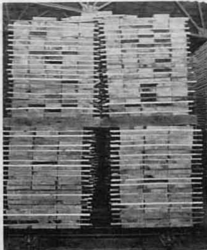
Above—Unit stacking on kiln trucks has been tried at Clearwater to determine if it is possible to satisfactorily season lumber so piled. Clearwater kiln foreman Phil Reinmuth thinks it may work okay.
