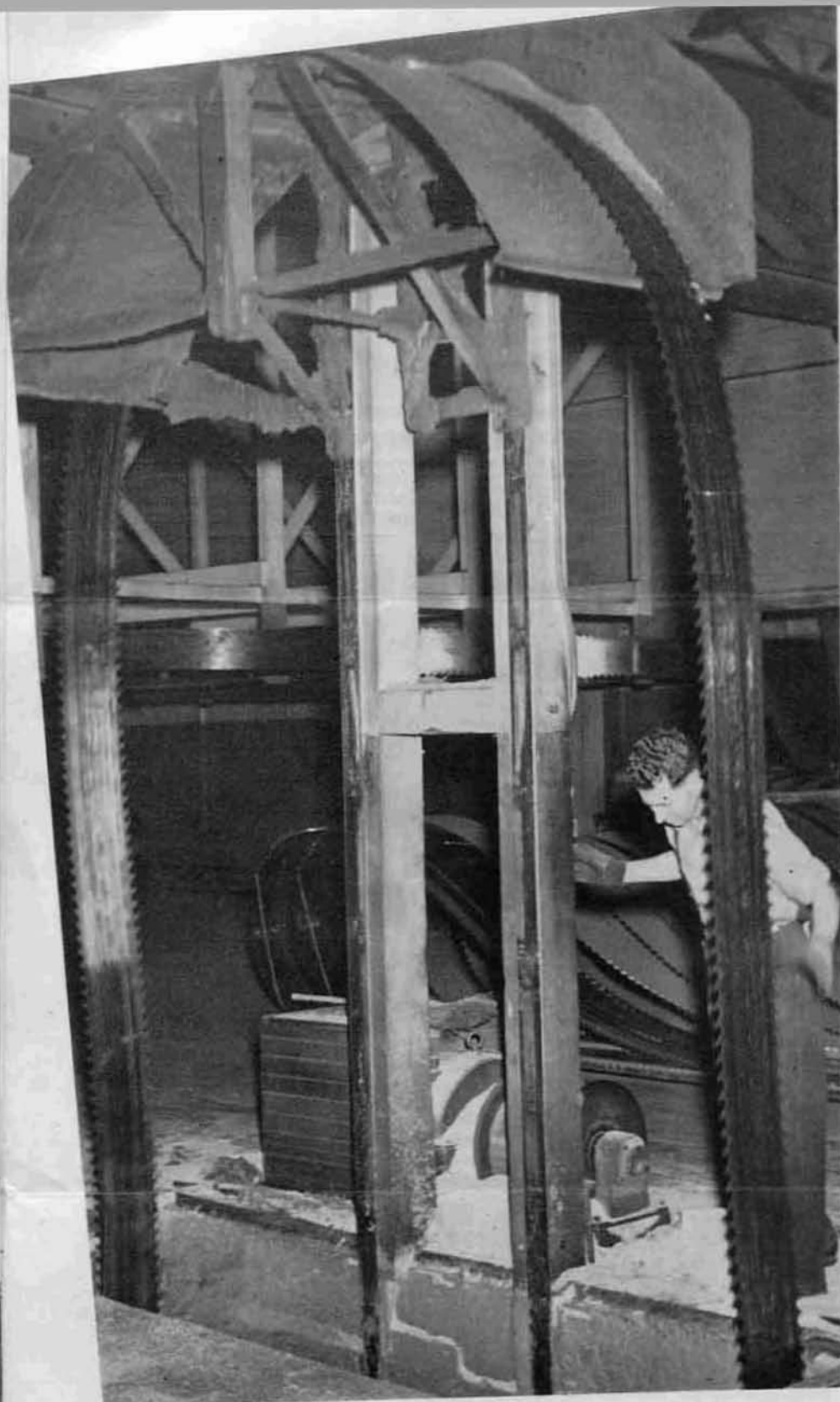
Above—Filer Miles Green carefully lowers a sharpened saw that will take its place over the band wheels and will be ready to cut lumber within four minutes of the time a change of saws was ordered.
