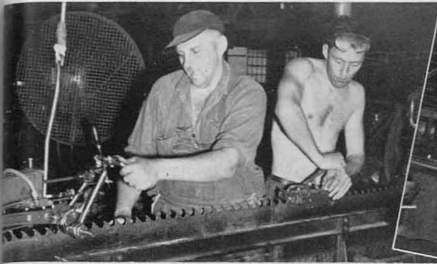
Above—Dick Vanator using the air swedge with Bill Bourasa on the shaper . . . Right—Bourasa using heat tension torches which are mounted above saw so that flame hits below each tooth on both sides.
