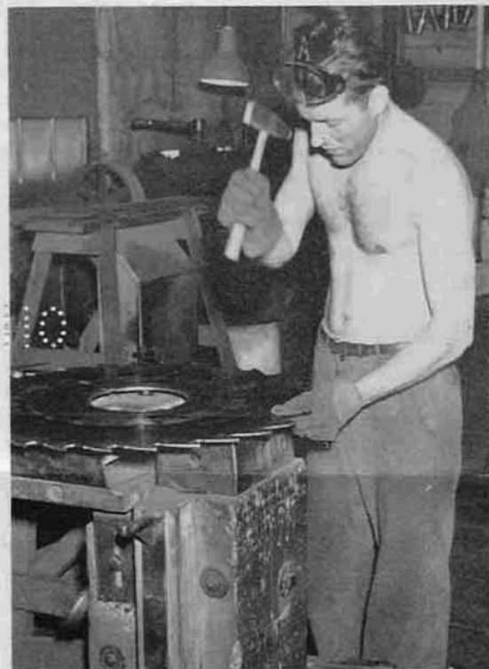
Above—The trusty hammer with which filing room dentists condition their patients . . . here ready to tap one of the 211 circular saws that are the particular responsibility of Filer Bill Bourasa. You might mistake this for a blacksmith shop scene, but it's only a conditioning measure. Diameters of circulars vary from eighteen to ninety-six inches.
