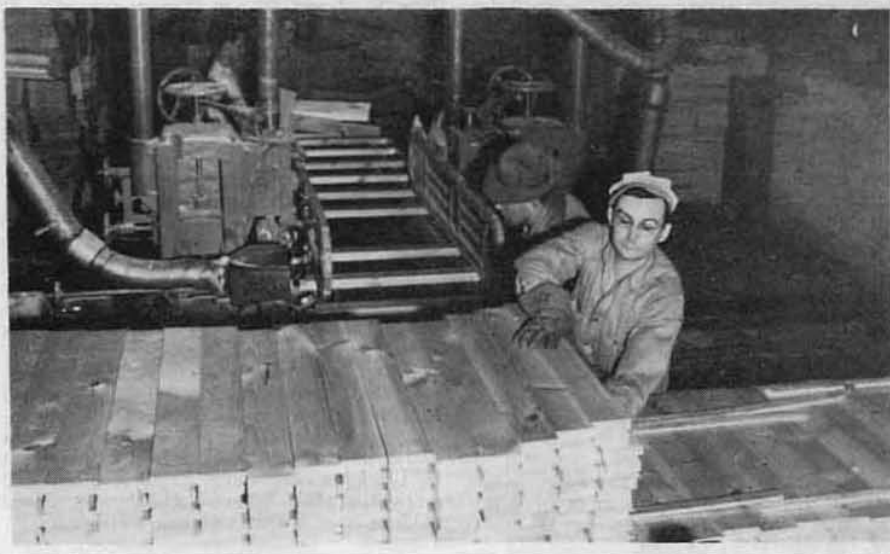
Above—Cutting lumber to exact length in a new department at Clearwater. Industrial orders for lumber of any exact length are handled here. The saws which operate from a foot control lever are several feet above the level of the plant floor. Cut-to-length pieces flow downward and away. Below—Stacking pieces of cut-to-order stock in the Clearwater Box Factory for the G-T-S Panel House.
