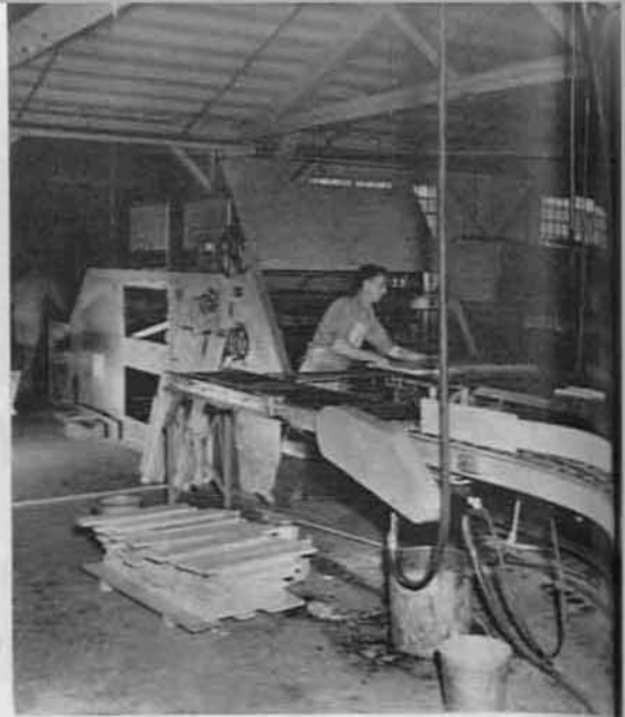
At left, four of the five cutoff saws in new cut-off department. At right, shows a picture of the electronic glueing machine.
