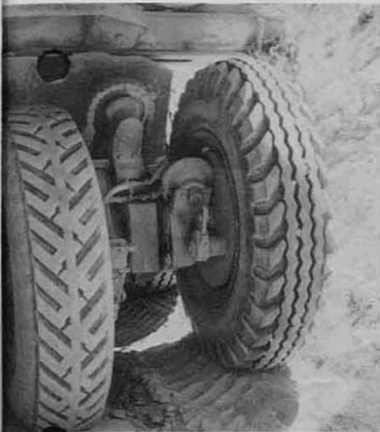
Above—Big load of logs from Camp 58, McComas Meadow. In hugging the bank on a corner the driver has the outside wheels at a higher elevation than the inside wheels but the compensator keeps the load evenly distributed on the tires . . . note the right rear wheels of the truck—light can be seen under one tire and the outside tire is bearing entire load weight. This well illustrates point sought by Hyster Engineer Anderson that Hyster trailer eliminates strain ordinarily placed on tires when truck rounds curves or travels over rough ground
