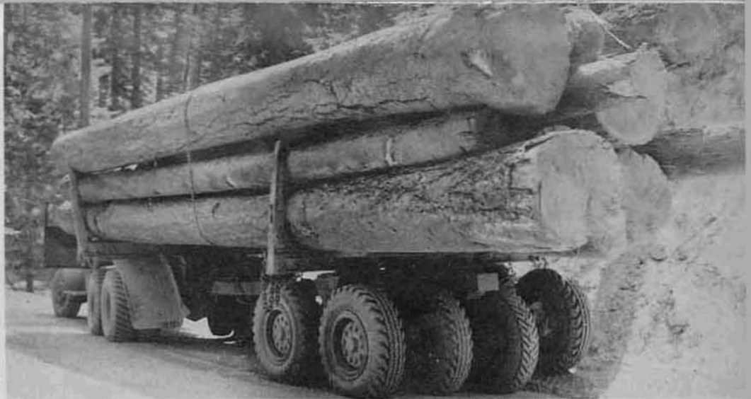
Above—Big load of logs from Camp 58, McComas Meadow. In hugging the bank on a corner the driver has the outside wheels at a higher elevation than the inside wheels but the compensator keeps the load evenly distributed on the tires . . . note the right rear wheels of the truck—light can be seen under one tire and the outside tire is bearing entire load weight. This well illustrates point sought by Hyster Engineer Anderson that Hyster trailer eliminates strain ordinarily placed on tires when truck rounds curves or travels over rough ground
