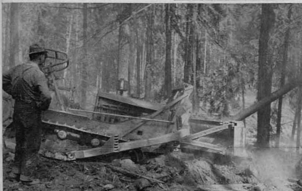
Below . . . a dozer in action making a fire trench around a blaze. Above insert shows the ravages of fire to our forests.
