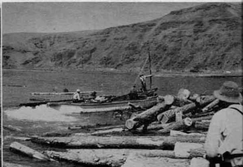
River boat churning water as it pushes logs from jam to fast current.
