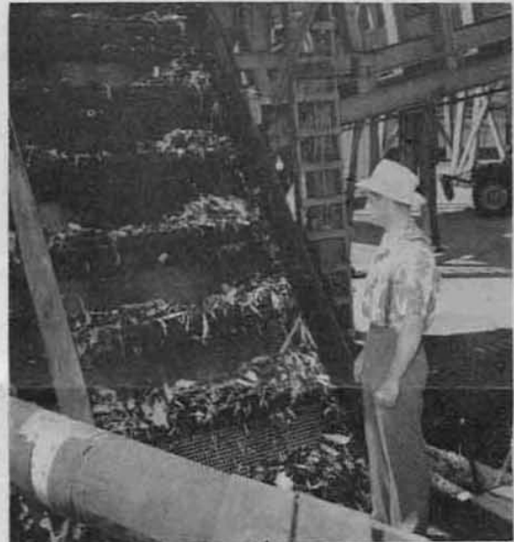
Below: Closeup of inclined screen which removes large chunks of bark from hydraulic barker refuse water. Engineer Frank Sule at right.
