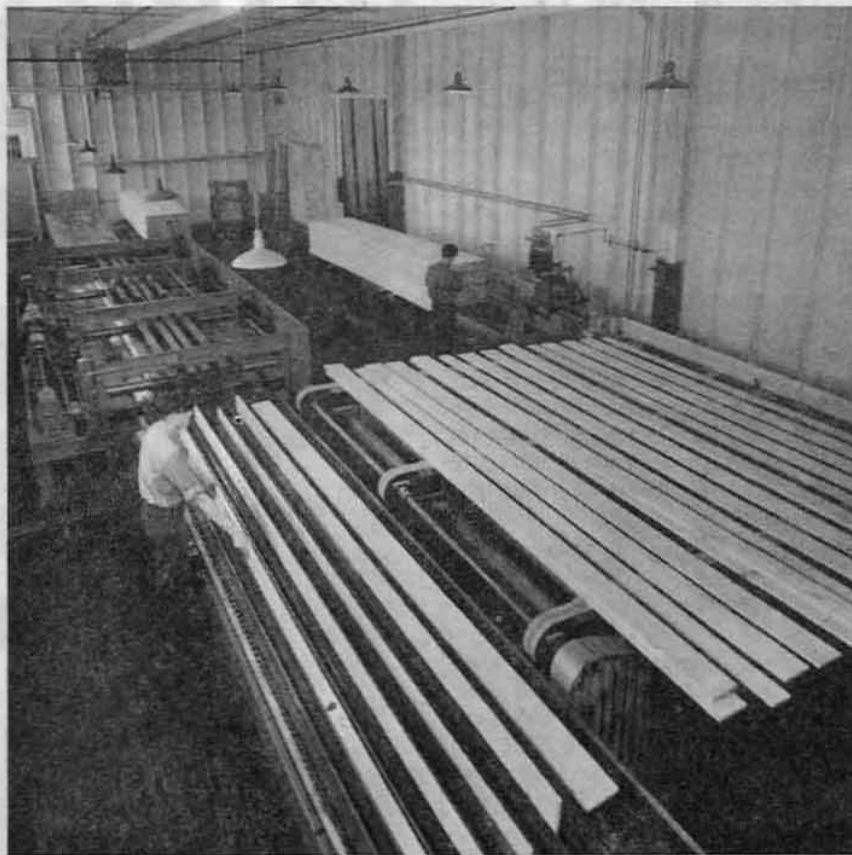
Narrow widths of Genuine Idaho White Pine receiving the synthetic resin on edges to be joined, which operation will take place in the machine in the background of this picture. (See story starting on page one.)
