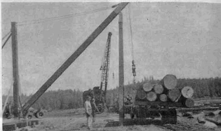
Above is a full view of the new unloader at the Potlatch pond which was designed and constructed by R. E. Owens, foreman of maintenance and construction at that unit. Besides being a time-saver it has a safety factor that keeps truckers out of the path of falling logs, the operation of the unloader being a push button device at a safe distance from the load.
