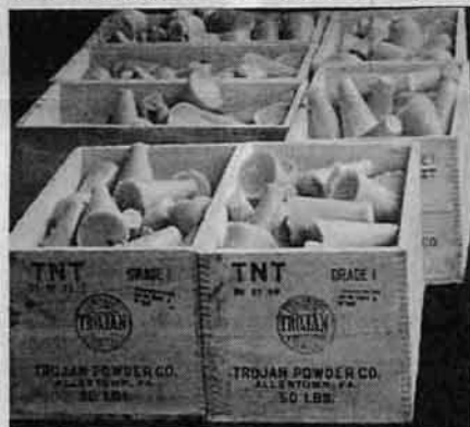
Wooden boxes of lock corner construction are used for TNT containers. Solidified TNT has the appearance of maple sugar.
