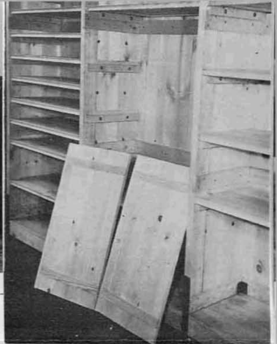
Assembled section of parts bin
