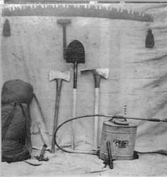
Fire tools—the crosscut saw, axe, pulaski and shovel are most frequently used.
