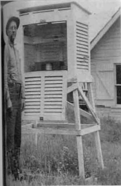
P.T.P.A. Warden RAY WOESNER has a look at the hygrothermograph that keeps a continuous record of temperature and humidity.
