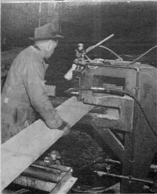
Feeding lumber into knot sealing machine—operator COY ALLEN, off-bearer, JOHN SOLBERG.
