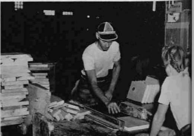
Below—Kenneth Dehnert and Jean Hanson at a rip saw. Dehnert is called a ripper and off-bearer Hanson is said to be "punking." It is her job to catch the various pieces ripped to a size that forms the correct width for the shook being made, then to stack them neatly on one of the box factory trucks on her side of the saw line. Dehnert feeds the saw and the speed with which he and other rippers do so determines box factory production in large part.
