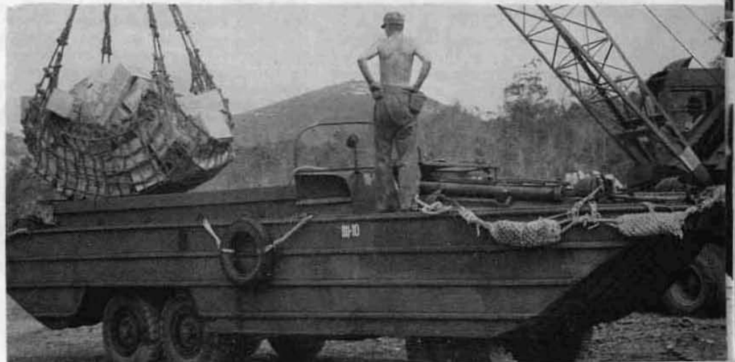
At a port-less Island in the South Pacific the Army takes supplies ashore in an amphibious truck. Supplies are lowered into the truck in a sling, are left in the sling to save time in getting "Duck" away from ship's side and in unloading ashore. Boxes are of a kind manufactured by P.F.I.
