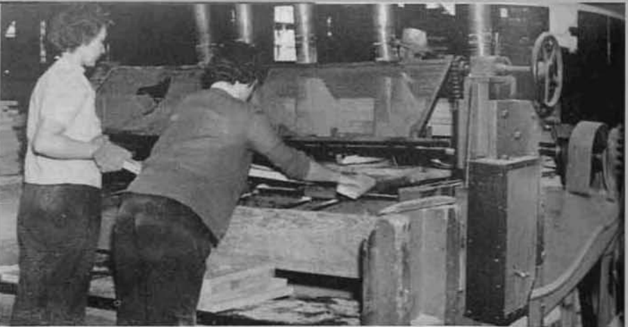
Above—Delores Tigges and Constance Sheneman at work on the equalizer, which in effect is a collection of cut off saws into which boards from the small planer in the background are fed by E. F. Triplett, standing between equalizer and planer.
