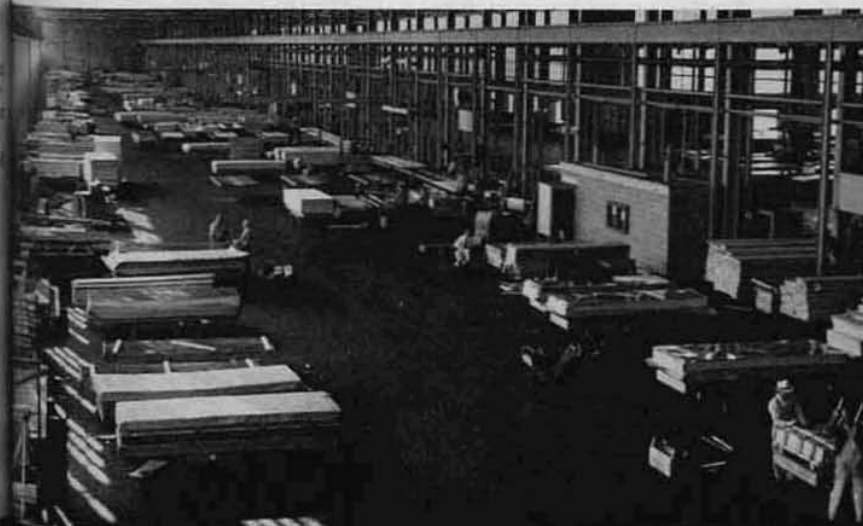
Below—West end of shipping area where sheets are interleaved and stacked for boxing. Paper is used between sheets to prevent scratches on the metal and water repellent paper used to protect the metal against water staining. A loaded skid of aluminum will weight up to 10,000 lbs.
