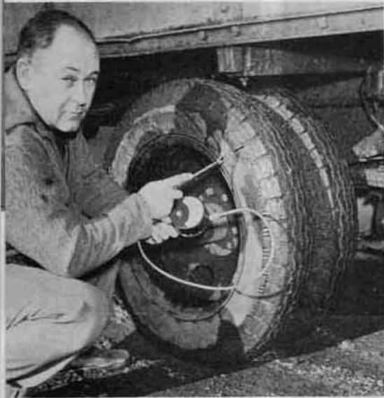
Tire Doctor John Huff makes use of the pyrometer to determine internal time temperature.
