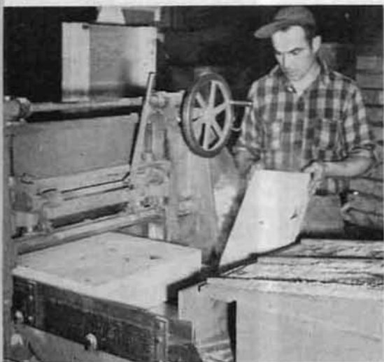
Above—Jack Byrnes, slicing machine operator, places another White Fir block on the feeder table. Slicer will cut 225 pieces a minute.
