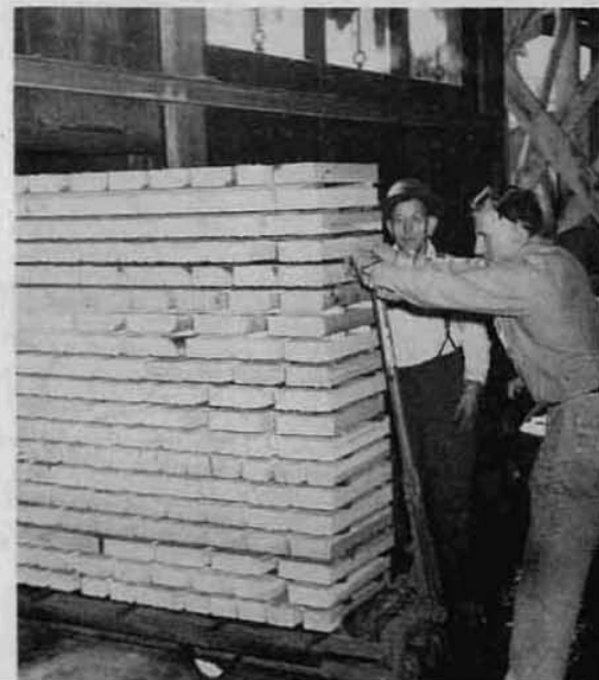
Below—Atkinson and Keiper push a load of blocks into one of the steam boxes.
